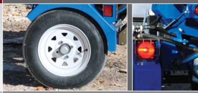
Hit the road in confidence with the easy trailing features that include Torflex® suspension axles, highway signal lights and 12-inch tires. The compact design folds together tightly, taking up minimal storage space.
