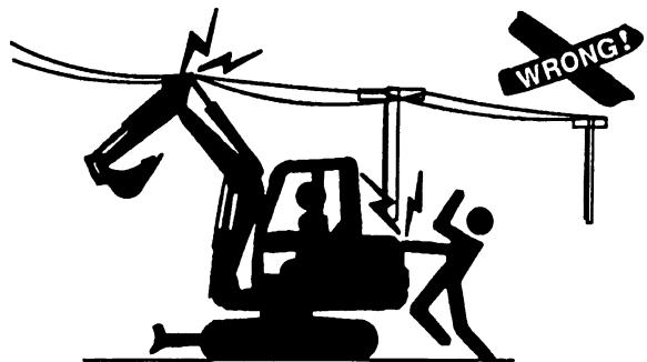
Electrical shock / electrocution
