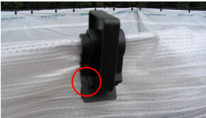
Picture 4: The top clip is closed securely when the outer section is completely pulled over the barbed hook of the inner section.
